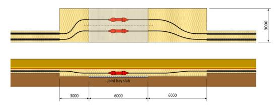
Figure 4.12: Typical Joint-Bay Dimensions (source: WSP | not to scale)
