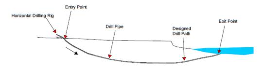
A small diameter pilot hole is drilled from the entry point, under the sea bed, to the exit point.
