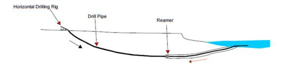
Next, a reaming tool is pulled back through the pilot hole to enlarge the hole. More than one pass may be required to make the hole larger than the diameter of the pipe
