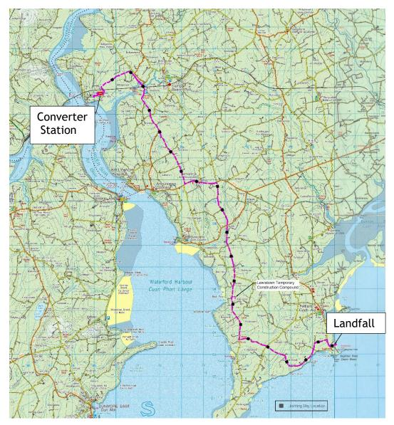
Figure 4.11: provisional Jointing Bay Locations | not to scale
