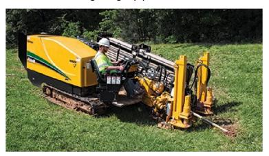
Figure 4.10: HDD Mini-Rig
