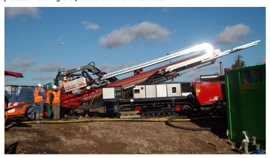
Figure 4.7: Photo of Typical maxi-rig HDD Drill Rig
